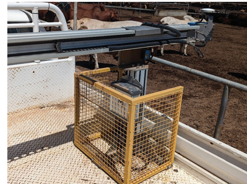
Figure 1: Tey's Australia Condamine Feedlot Bunk Scanner in service, installed on tray of site's bunk calling ute.
